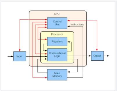
Block diagram of a basic computer with uniprocessor CPU. Black lines  $^{65}$  indicate data flow, whereas red lines indicate control flow. Arrows indicate the direction of flow.
